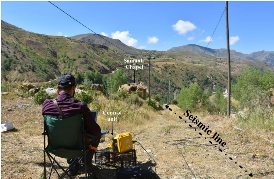
Figure 4. Seismic refraction and MASW methods line direction measurement layout
