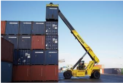
Figure 8(a). Container Reach Stacker (CRS) (Hyster, 2023).
