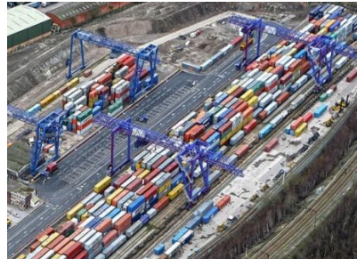
Figure 3(b). Rail Mounted Gantry (RMG) (Liebherr, 2023b).
