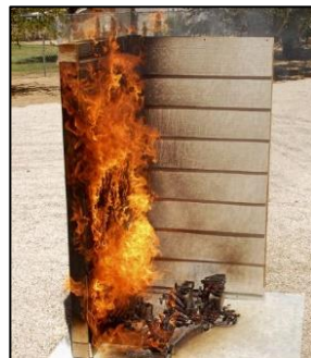
Figure 13-14. Flame penetration (burn through) at the rabbeted bevel lap joint in a solid wood siding product, as viewed from the stud cavity side of the wall (Left).Flames from the fire would have impinged on windows and eave, if they had been present (Right).(Quarles et al., 2010)
