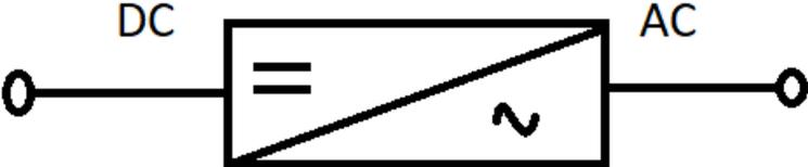
*Figure 1. Inverter general structure*
