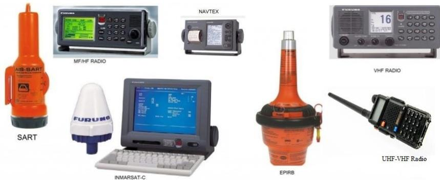
Figure 4. *Communication Equipment on Ship (Marinegyaan, 2023)*
