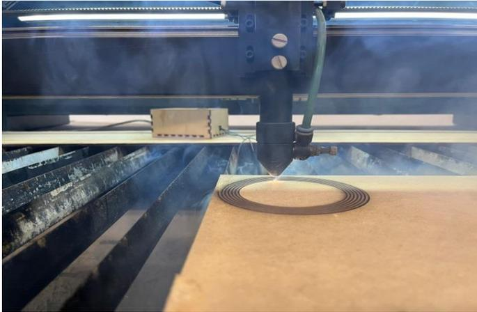
*Figure 5. Processing of MDF plate with CO<sub>2</sub> laser cutting device*
