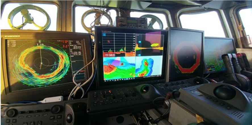
*Figure 10. Sonar and Echo Sounders (Hydro International Magazine, 2023)*
