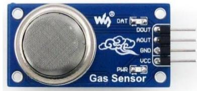
*Figure 3. MQ-7 carbon monoxide gas sensor*
