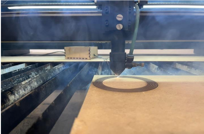
Figure 5. Processing of MDF plate with CO 2 laser cutting device
