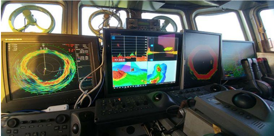
Figure 10. Sonar and Echo Sounders (Hydro International Magazine, 2023)
