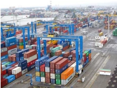
Figure 3(a). Rubber Tyred Gantry (RTG) (Konecranes, 2023b).
