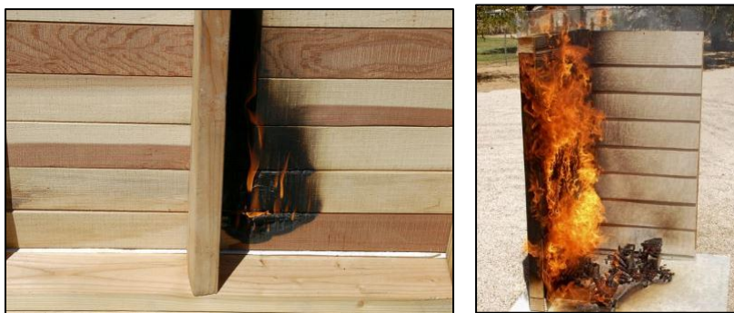
Figure 13-14. Flame penetration (burn through) at the rabbeted bevel lap joint in a solid wood siding product, as viewed from the stud cavity side of the wall (Left). Flames from the fire would have impinged on windows and eave, if they had been present (Right). (Quarles et al., 2010)
