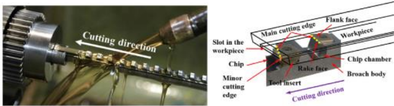
Figure 6 Application of the Single Broach method and pen sections (Huang et al. 2023)
