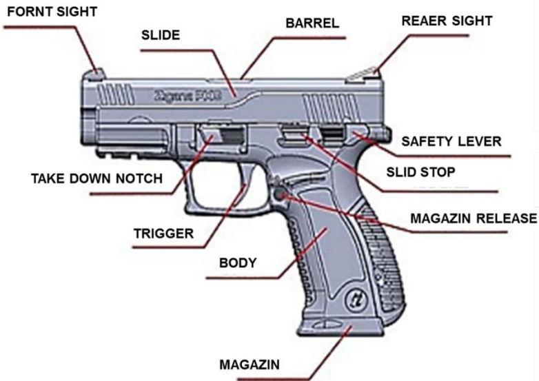
Figure 1. General parts of a firearm (Guner 2019)
