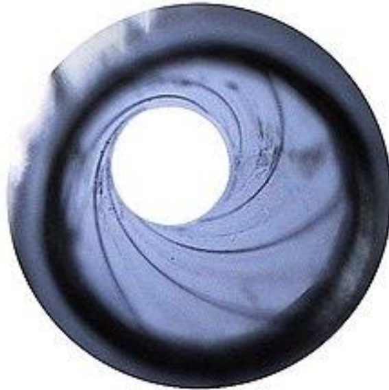
Figure 5 Image of the rifle-set structure of a standard pistol (2023c)
