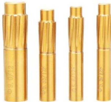
Figure 7 Cutting tool used in the button method (Guner 2019)
