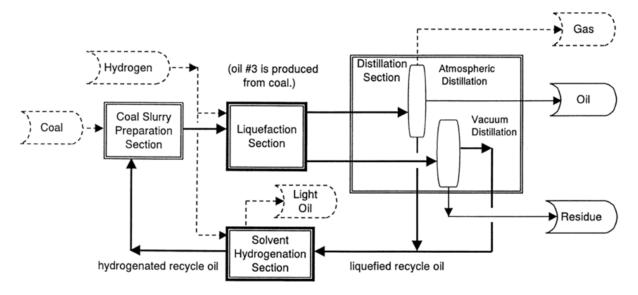
Figure 7. Schematic diagram of a typical direct coal liquefaction process (Ali & Zhao, 2020)
