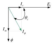
Figure 8. Phasor diagram of excitation current
