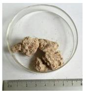
Figure 2. Visual analysis of mortar sample 1 in chemistry laboratory
