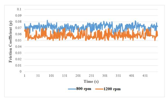
Graphic 1. Friction coefficient change of Etial 171 sample with 10W40 oil at 800 and 1200 rpm.
