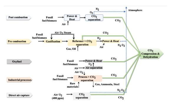
Figure 4. The stages of carbon capture methods (Lau et al. 2021; Davoodi et al. 2023)
