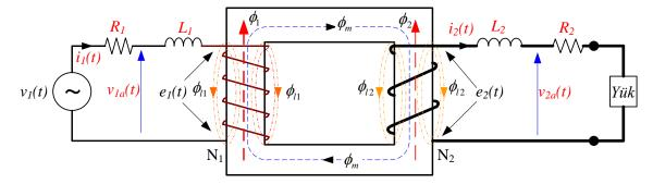
Figure 6. Model of a Transformer
