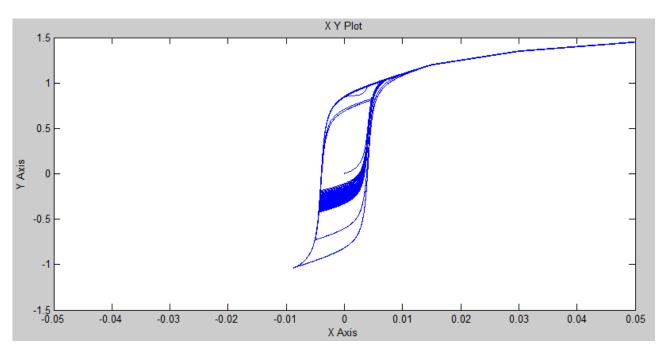
Figure 16. Hysteresis loop of the transformer under specified load and operating conditions.
