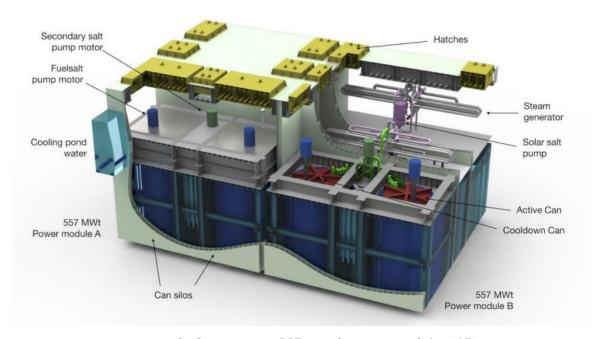
Figure 8 Thorcon Two 557 MWth power modules (17)
