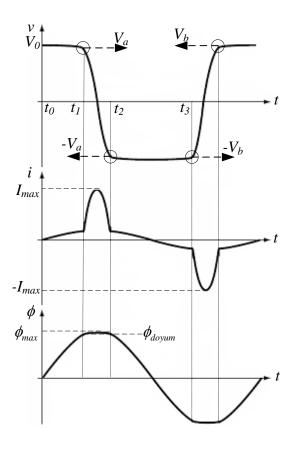
Figure 12. Time variation curves of capacitor voltage, series circuit current and magnetic flux in iron core inductance.
