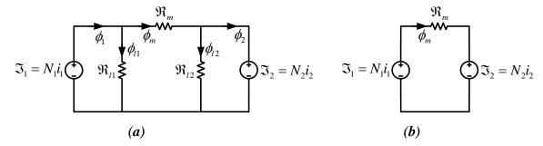
Figure 7. (a) Detailed magnetic equivalent circuit of a transformer (b) Equivalent electrical circuit
