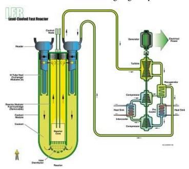
Figure 4 Lead cooled fast reactor LFR cycle (11)
