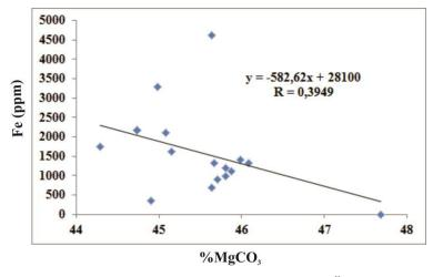
Figure 11. %MgCO<sub>3</sub>-Fe (ppm) graph (from Özkan, 2016)
