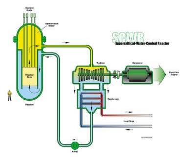
Figure 9 Supercritical-Water-Cooled Reactor (SCWR) cycle (11)
