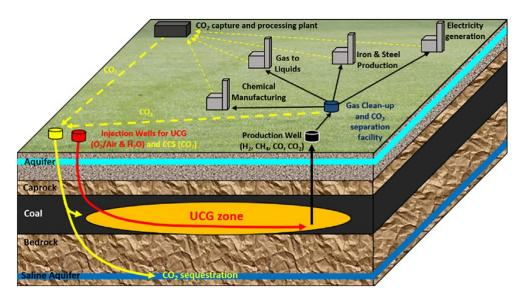
Figure 3. Underground coal gasification proces (Zagorščak et al. 2019)
