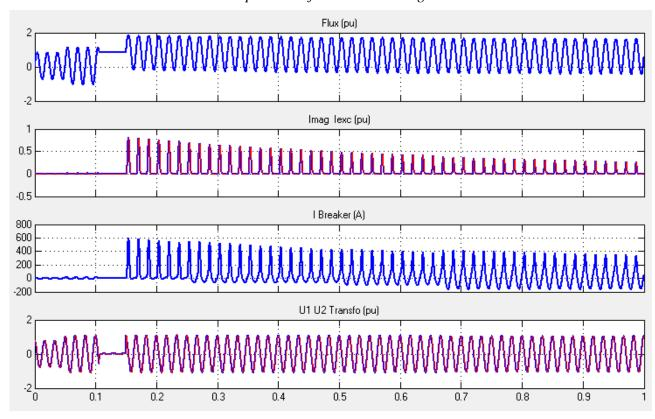
Figure 19. Change of electrical parameters during the process when the switch in the transformer primary changes position
