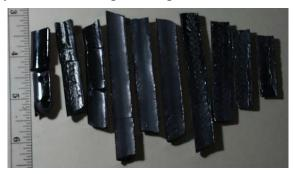
Fig. 2. Zone refined Se ingots (Oner, 2015a)
