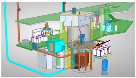
Figure 6 Schematic view of Chinese molten salt reactor (15)
