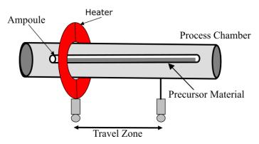
Fig. 1. The schematic of a generic zone refining setup
