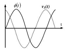
Figure 2. Variation of magnetic flux with voltage.
