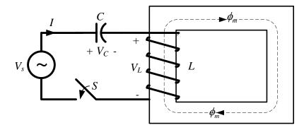
Figure 10. Connecting a coil wound to a closed magnetic circuit.
