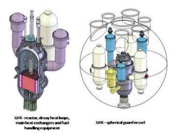
Figure 9 GFR reactor and guard vessel (11)
