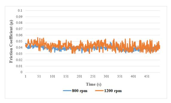
Graphic 2. Friction coefficient change of ETİAL 171 sample with 20W50 oil at 800 and 1200 rpm.
