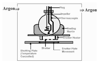
Fig. 3. Schematic of a generic a-Se alloying reactor (Chowdhury, Oner & Mandal, 2017)
