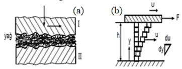
Figure 3. (a) Liquid Friction model and (b) liquid friction diagram (Hatice et al., 2020).
