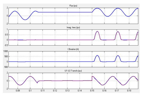
Figure 18. Detailed examination of the changes in electrical parameters during operation when the position of the switch changes
