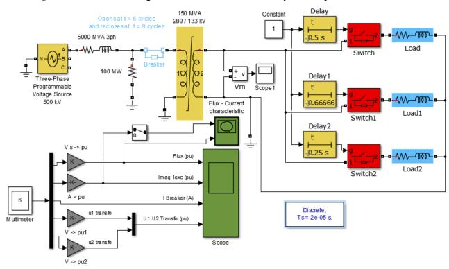
Figure 15.Block diagram of the installed system.
