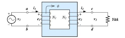
Figure 3. Load-Connected Ideal Transformer.
