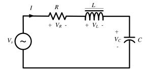
Figure 13. A ferroresonance circuit
