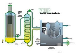
Figure 11 Very-High-Temperature Reactor (VHTR) cycle (11)
