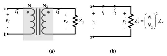
Figure 5. (a) An ideal transformer with a load connected to its secondary. (b) Equivalent electrical circuit.
