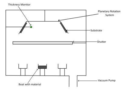
Fig. 5. Schematic of a generic Thermal Evaporation System
