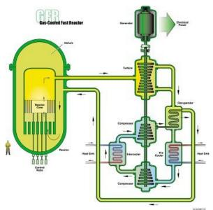
Figure 8 Gas-cooled fast reactor FR system representation (11)
