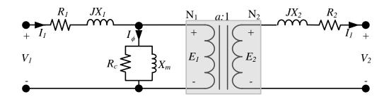
Figure 9. Equivalent circuit of a real transformer
