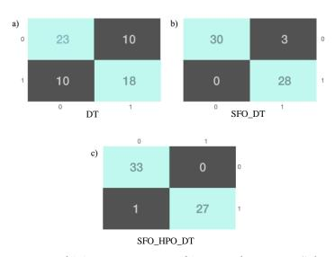
Figure 3. Confusion Matrix of (a) Decision Tree, (b) DT with Feature Selection, (c) Proposed
