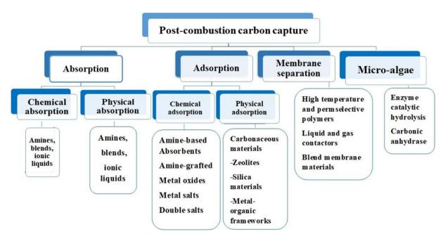
Figure 6. Post-combustion carbon capture methods (Osman et al., 2020)
