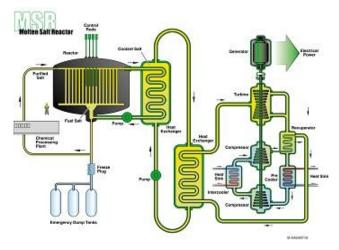
Figure 5 Molten salt reactor (MSR) cycle (11)
