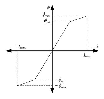
Figure 11. Simplified magnetic flux-current characteristic of a coil wound in a closed magnetic circuit
