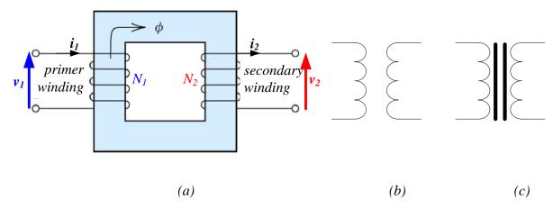
Figure 1. A transformer core and its symbols
