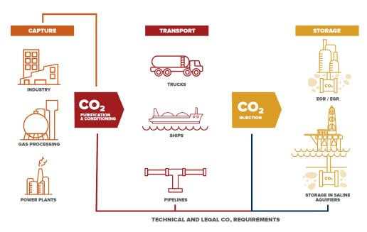
Figure 5. A framework for carbon capture, transport and storage processes (Kearns et al., 2021)
