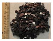
Fig. 4. A-Se alloy pellets (Oner et al., 2015a)
