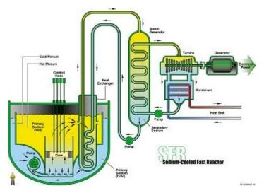
Figure 10 Sodium-Cooled Fast Reactor (SFR) cycle (11)
