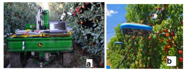
Figure 1 Unmanned ground vehicle (a) (Silwal et al., 2017), unmanned aerial vehicle (b) (Anonymous a, 2022)
