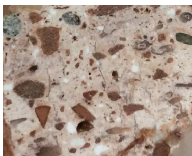
Figure 13. Thick section photograph of Sample 6
