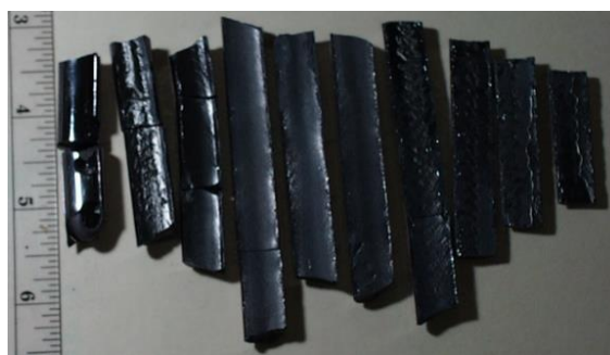
Fig. 2. Zone refined Se ingots (Oner, 2015a)
