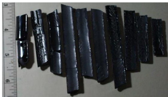
Fig. 2. Zone refined Se ingots (Oner, 2015a)
